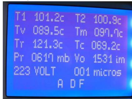
T1 temperatura sonda camera
